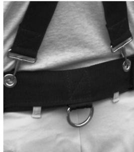
**Note:** There are two specially designed straps located at the back of the E-Z Swing belt. The straps use hook and loop material, and are designed to wrap around and lock the E-Z SWING belt in place on top of your own existing belt. The straps will help keep the belt in the most comfortable position when using the harness attachment.
